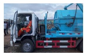
Photo: A skip loader operating a mechanical arm to lift and transport 5 m<sup>3</sup> garbage bins to landfill sites. (Photo by UNICEF, May 2017)
